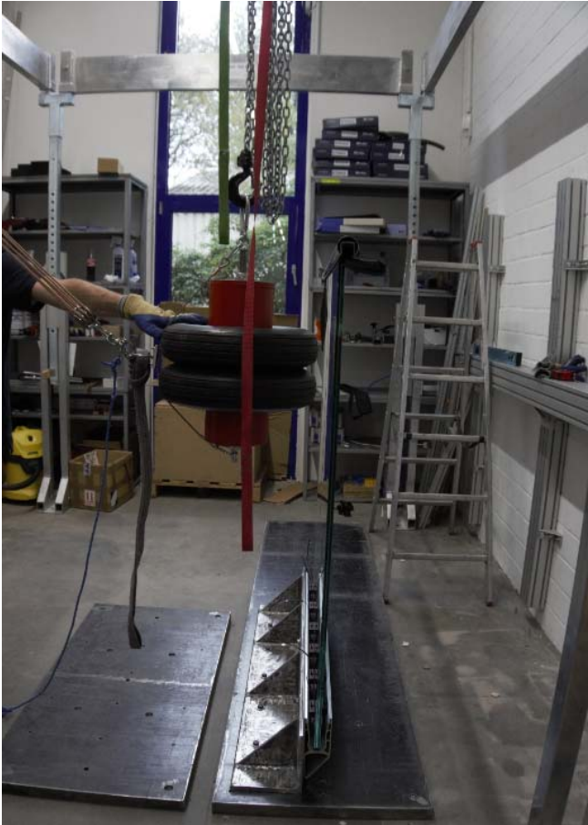
Image 21 Test setup for the impact test with twin-type impactor
