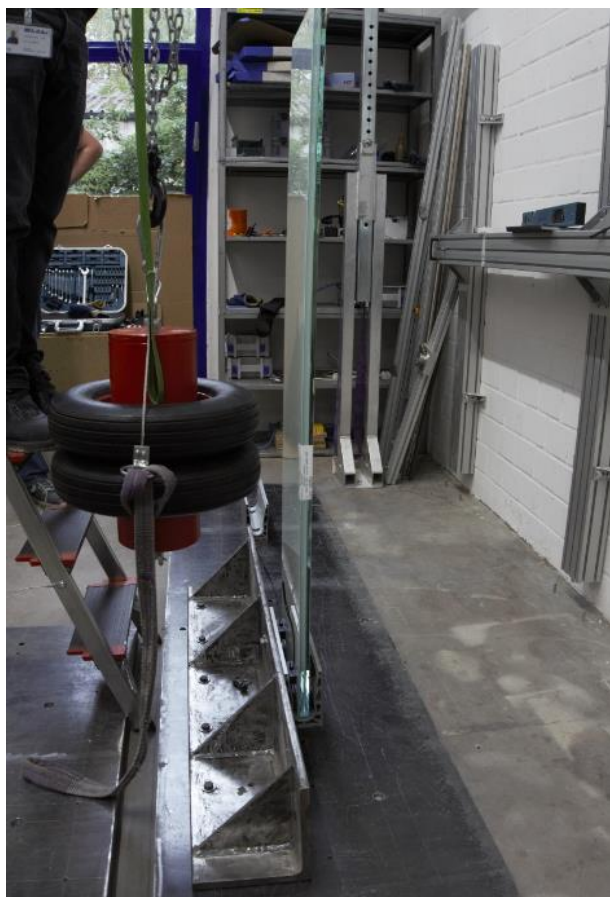
Image 25 Test setup for the impact test with twin-tyre impactor (for VetroMount Side)
