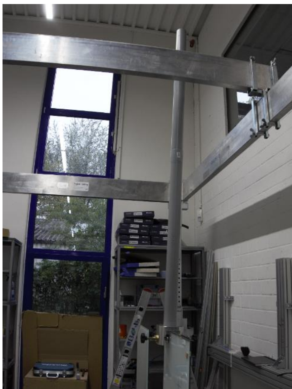
Image 22 Test setup for the hard impact test
